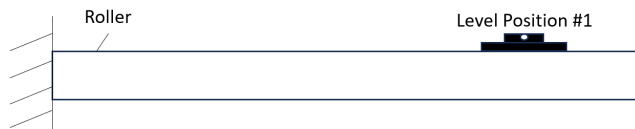
Diagram 3: Checking for roller deflection due to weight.
