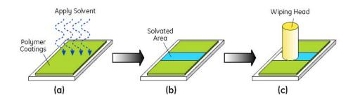
Figure 5 Low cost R2R compatible solvent-assist-wipe patterning technique for organic thin film. (a) Apply solvent to the to-be-patterned area. (b) Solvent dissolves the organic coating material in applied area. (c) Use a polymeric wiping-head to physically remove organic material.
