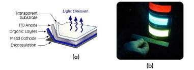
Figure 1 (a) Schematic of an OLED device. (b) Flexible red, blue, and green OLEDs.
