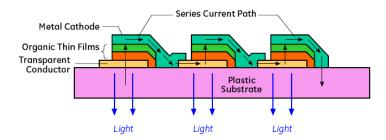
Figure 2 Fault tolerant monolithic series device architecture for large area OLEDs.
