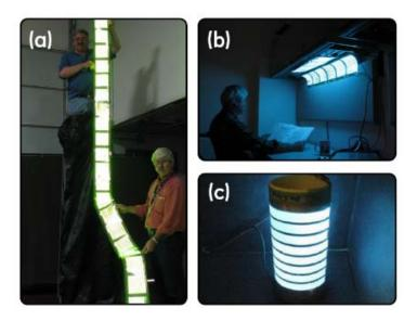
Figure 4 (a) 15 feet long green R2R OLEDs. (b) Under cabinet light made from blue R2R OLEDs. (c) Blue R2R OLED wrapped around a three-inch-diameter plastic core.
