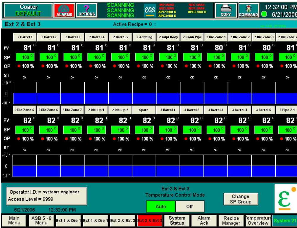
Figure-2: Barrel & Die Zones Temperature Control Display integrated into the on-line Web gauging system
