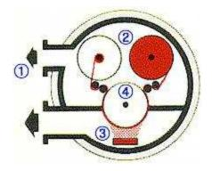
The rolls in a vacuum metallizer must be parallel within a certain tolerance or wrinkles will occur in the metallized plastic film. Wrinkles in the plastic film often result in the product becoming non-recyclable scrap which is costly.
