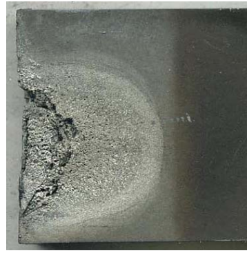
Fig. 9 Damaged and clipped edge of the boat applied in the measurement of Fig10.
