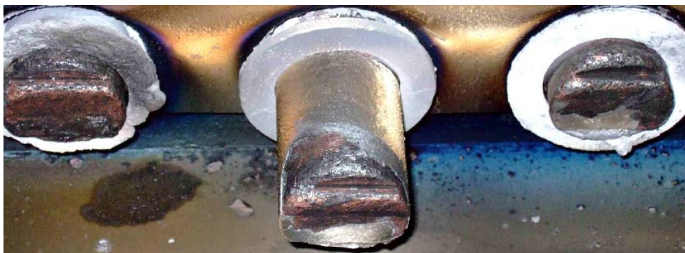
Fig. 1 Electrodes eroded after long time evaporation
