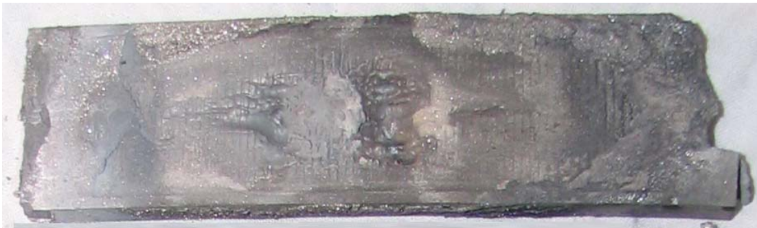
Fig. 4 Eroded boat edge was finally chipping or broken down
