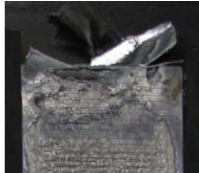
Fig. 2 Small crack appeared at a boat edge Fig. 3 Eroded boat edge by localized heating
