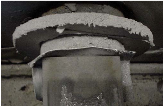
Fig. 2 Small crack appeared at a boat edge Fig. 3 Eroded boat edge by localized heating
