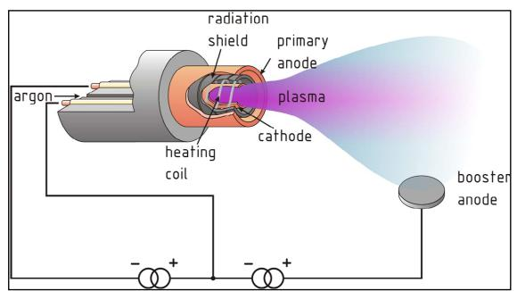
Figure 4: Section view of the plasma unit.
