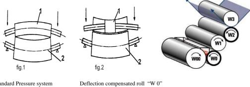
The pressure on to the rolls can be guaranteed over the complete
