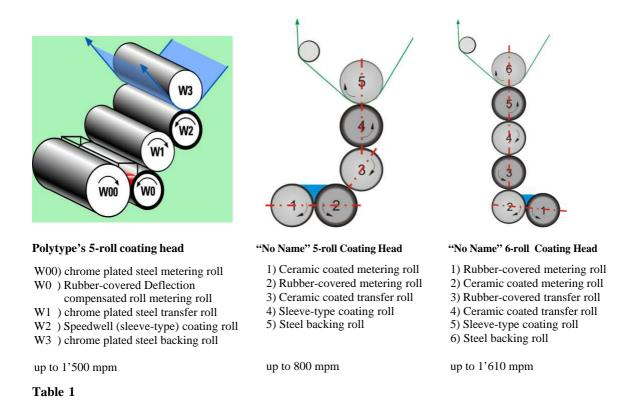
By focusing on the parameter "speed" only one will ask why does Polytype's 5-roll coating head, with its technical solution, allows and achieves what a 6-roll coating head is offering in comparison.
