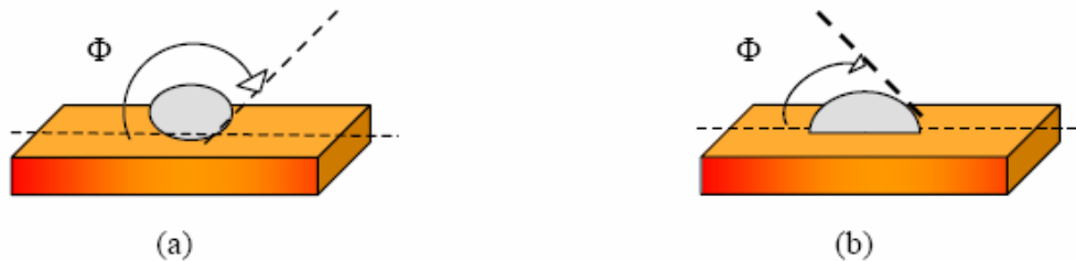
Figure 2. Contact angles representing two cases of boat wettability by molten metal: (a) poor wetting boat and (b) good wetting boat
