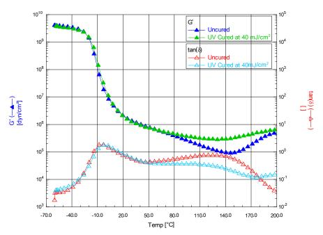
Figure 10. Temperature Dependence of G' and  $tan(\delta)$  for PSA
