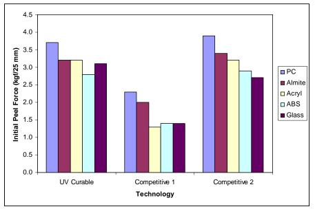
Figure 11. Peel Adhesion on Various Substrates
