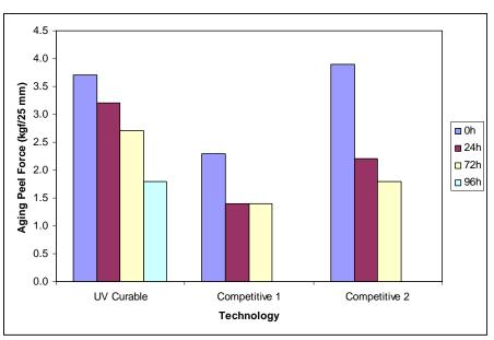
Figure 12. Resistance to Aging at 80°C & 85% RH
