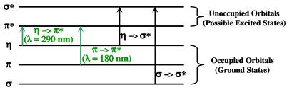
Figure 3. Electronic Excitation of C=O in Acrylate
