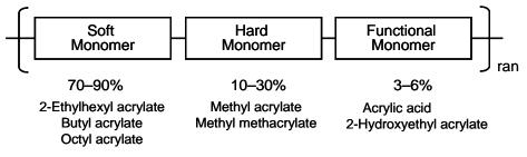
Figure 2. Typical Acrylic PSA Polymer Composition
