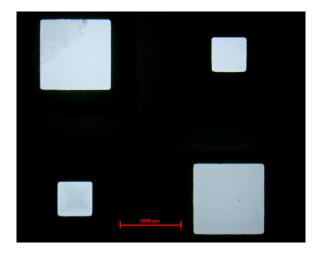
Figure 3. The image shows 4 quadrant layout on a  $35 \times 50$  mm<sup>2</sup> aluminum sheet during an electrical test. The first HTL thickness maximum fabricates good yield data on the aluminum test sheets of around 70 - 80 %, but not sufficient device stability.
