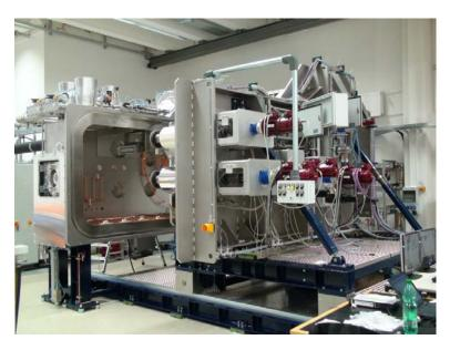
**Figure 6.** A photograph of the roll-to-roll coater with the open process chamber.
