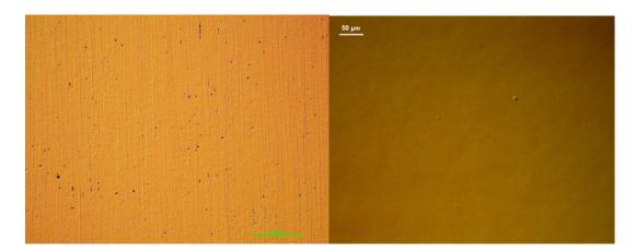
Figure 1. Optical images of surfaces of an untreated aluminum foil with a non-conducting smoothing lacquer and not cleaned, see left image. The right image shows the same type of aluminum foil, but cleaned and coated with silver. The left image shows clearly the texture
