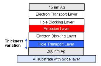
Figure 2. A principle design of a pin OLED stack.
