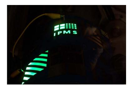
Figure 1. The photograph shows a green OLED deposited aluminum sheet under electrical testing. Power efficiencies between 20 - 25 lm/W is well possible for green pin OLED stacks on aluminum sheets (for comparison: A 75 W filament lamp has  $\approx 12 \text{ lm/W}$ ).
