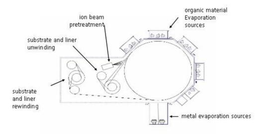
Figure 2. Schematically drawing of the roll-to-roll vacuum coater with the 2 m diameter sized deposition cylinder with the arranged deposition modules.
