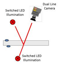
Scan rate synchronized light switching technology, one of the most recent innovations few systems master, provides simultaneous acquisition of the sheet at multiple illumination modes with a single bank of cameras which significantly increases detection and classification performance without the traditional high cost of multiple camera banks.
