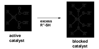
Since aliphatic laminating adhesives are significantly used in food packaging, most of the testing included raw materials with FDA compliance and low-to-zero extractability. The blocking agents included in this paper are a monofuntional mercapto-silane and a trifunctional mercaptan. The catalyst is dibulyltin dilaurate.
