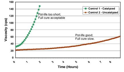
Figure 1. Initial viscosity profiles of current aliphatic isocyanate laminating adhesives.
