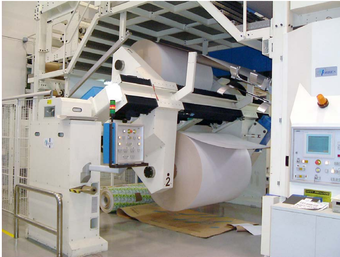
Figure 8 – MTorres turret splicer circa 2010 - this photograph will be used to show the differences when compare Figure 7 the Floor Pickup design.
