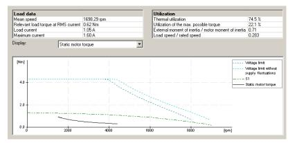
Figure 7: Motor Selection / Load Requirements
