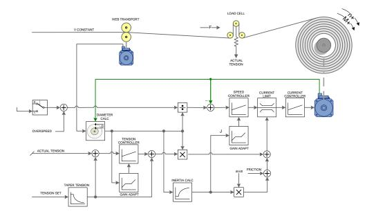
Figure 2: Torque Limiting Control (with load cell sensing)
