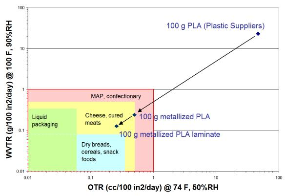
Figure 5: High Barrier Metallizing on 100 g PLA Film
