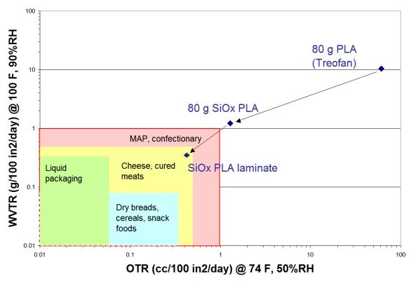
Figure 4: SiOx-coated Clear Barrier on 80 g PLA Film
