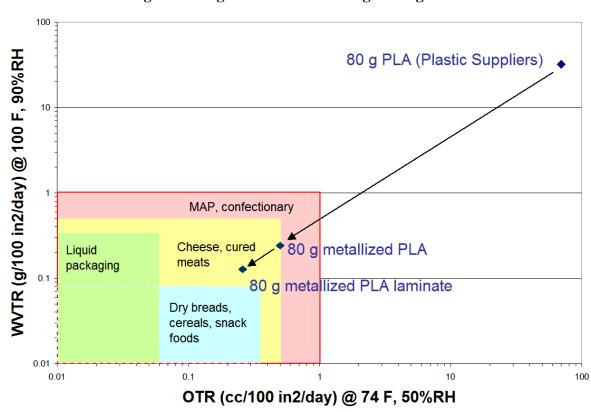
Figure 6: High Barrier Metallizing on 80 g PLA Film
