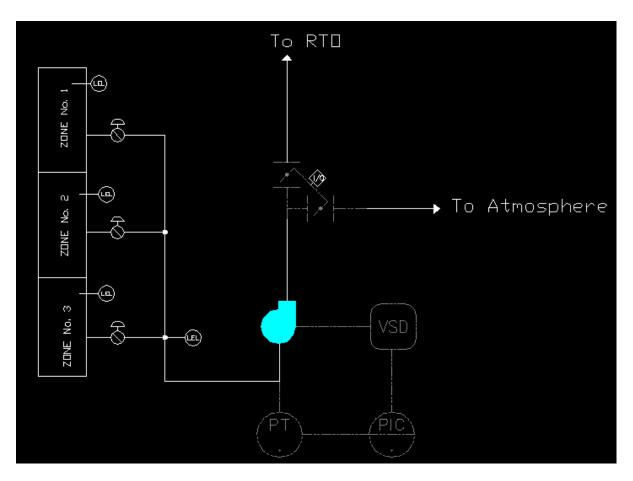
The second area of benefit is the exhaust systems for the individual lines, these coupled with T-dampers provide flexibility to the operation.
