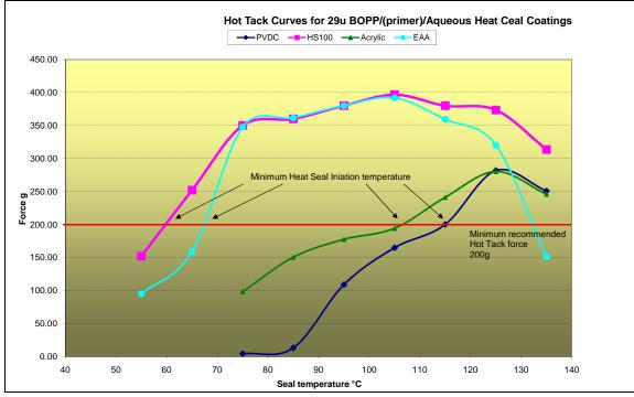
Figure 2 Primerless Heat Seal Coating Compared to Conventional Coatings
