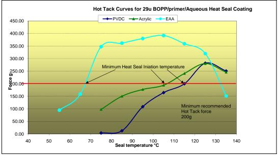
Figure 1 Hot Tack Data For Conventional Heat Seal Coatings
