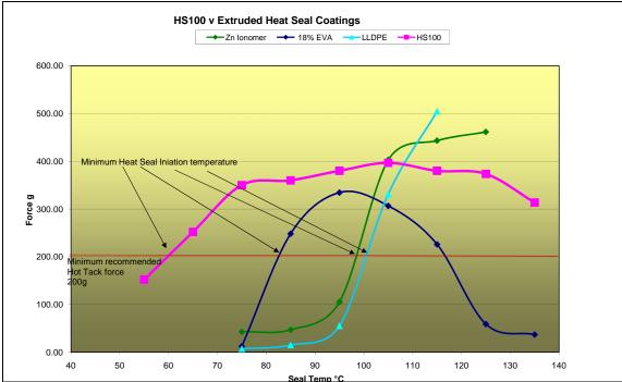
Figure 3. Comparison of Aqueous HS100 Heat Seal Coating to Extruded Sealant Resins
