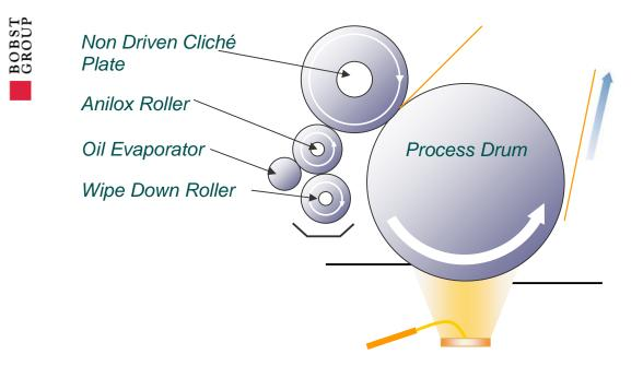
Figure: 3.0 A simplified schematic to illustrate a pattern printing system
