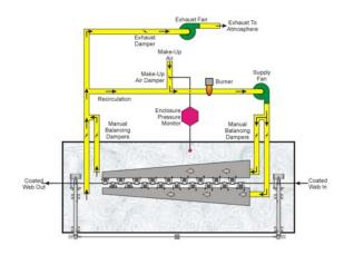
Fig. 2. Tapered air distribution header
