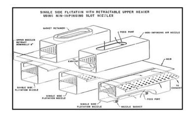
Fig. 6. Single side flotation nozzles combined with dilution air bars.
