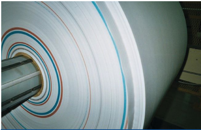
FIGURE 4. A roll which has been marked with an ink edge-marking system. With edge markers, the entire defective section of a roll can be marked.
