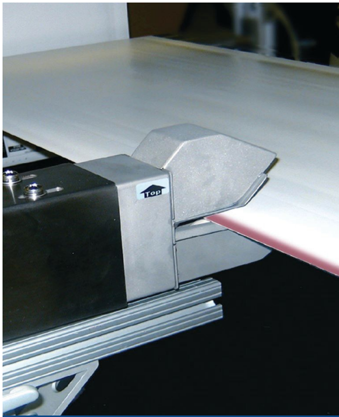
FIGURE 3. Edge-marking systems spray ink to mark the location of defects. Multiple markers with various colors can be used to distinguish defect categories.
