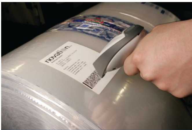
FIGURE 5. The roll-map data is printed on a label placed on the finished roll. The 2D barcode contains all the data and can be scanned in at the subsequent process to automatically stop the line at the defective locations.
