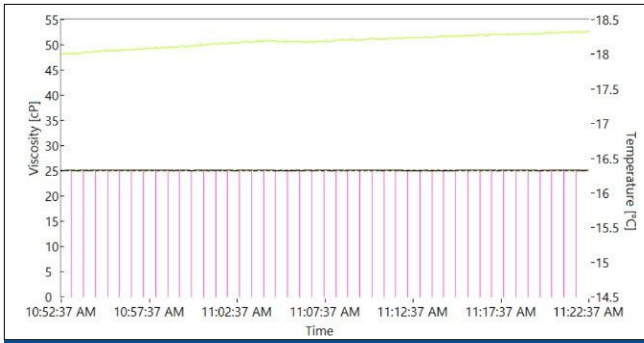
FIGURE 9a. Temperature-compensated viscosity (black, 25cP) and temperature (green, ~18° C) vs. time, coarse vertical scale
