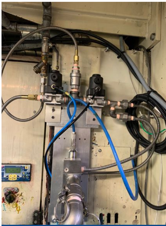
FIGURE 7. Viscometer installed using a flow adapter, showing the control valves for precise dosing of solvent to regulate ink viscosity.
