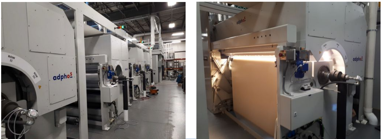
FIGURE 1. A gravure-printing press (left) equipped with aNIR technology (right) for drying water-based inks and varnishes.
