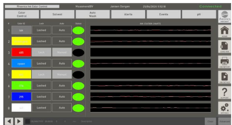
FIGURE 8. Interface screenshot showing an 8-station gravure press with six stations active
