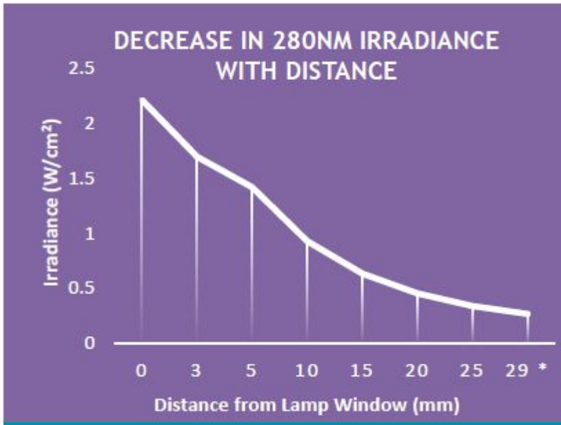
FIGURE 2. Irradiance-distance decay for 280-nm UV-LED lamps. The maximum adjustable height for this test = 29 mm.
