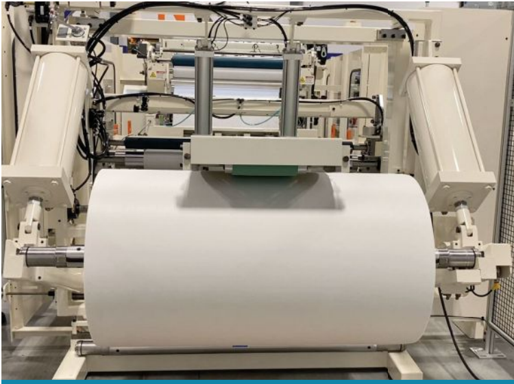
FIGURE 1. Master roll unwinding section of the automatic perforator-rewinder system
